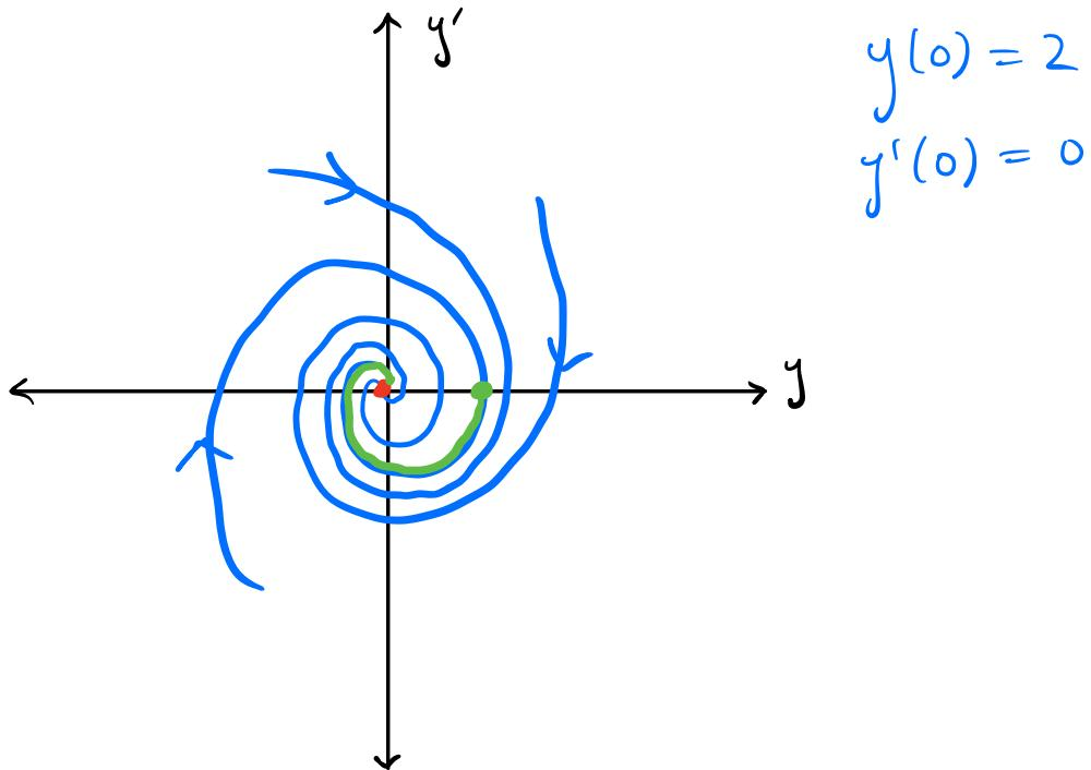
Notice that all of the solutions to this ODE oscillate. We say that this spring-mass system is underdamped.
