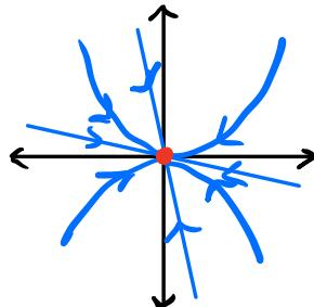
$$\textcircled{2} \quad \underline{\gamma^2 = 4mk} \quad \rightarrow \underline{\text{degenerate sink}}$$
