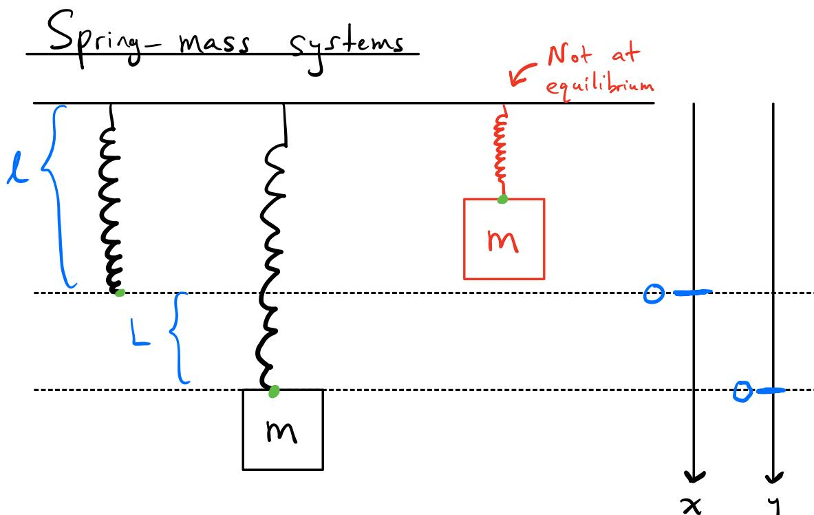
$$x = \frac{\text{displacement from spring's natural length}}{\text{length}}$$
