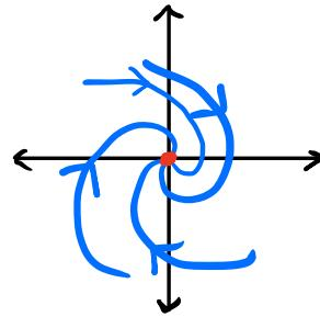
Notice that only in case  $\textcircled{3}$  do we see solutions which oscillate. If  $\underline{\gamma < 2\sqrt{mk}}$ , we say that our spring-mass system is underdamped.
