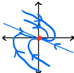
$$\textcircled{3} \quad \underline{\gamma^2 < 4\sqrt{mk}} \rightarrow \underline{\text{Spiral sink}}$$
