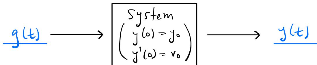
Of course, the output  $\underline{y(t)}$  doesn't just depend on the input  $\underline{g(t)}$ . The system will have some response to the initial conditions, even if no forcing is present.
